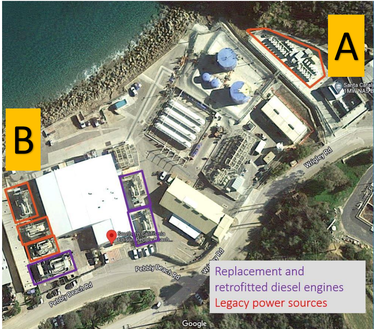
Figure 2-6: Land Availability at the Electricity Generating Facility Located on Santa Catalina Island
