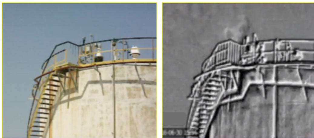
Figure 2-1: View with naked eye compared to view with an OGI camera
