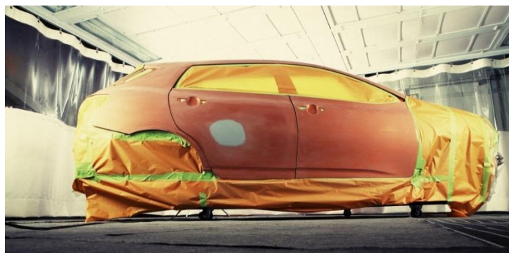
Figure A5c-3: Auto Body Repair Shop Painting a Motor Vehicle
