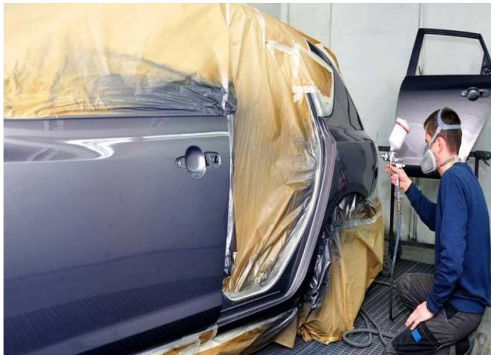
Figure 4-13: Application of Automotive Coating Inside a Paint Spray Booth
