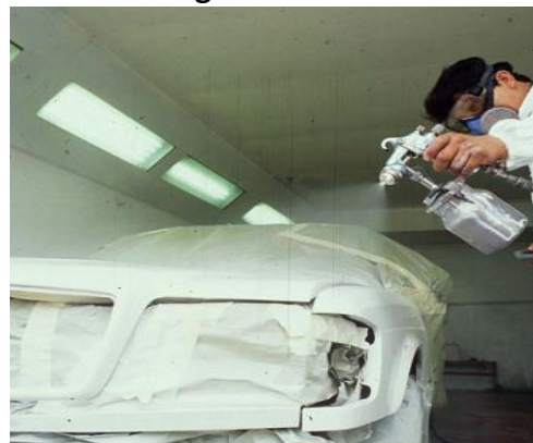
Figure A5c-2: Auto Body Repair Shop Painting a Motor Vehicle
