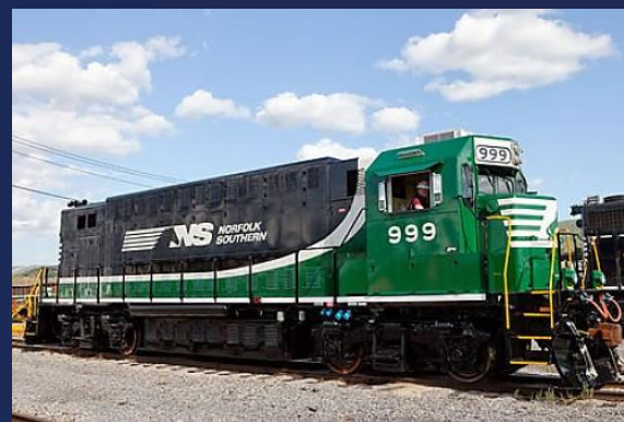
Battery electric switcher locomotive
