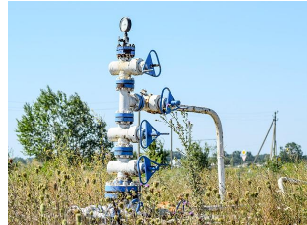
Example of an Injection Well
