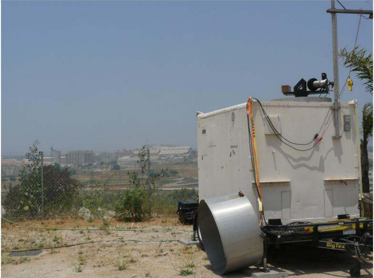
Figure 1 Lidar system overlooking cement plant
