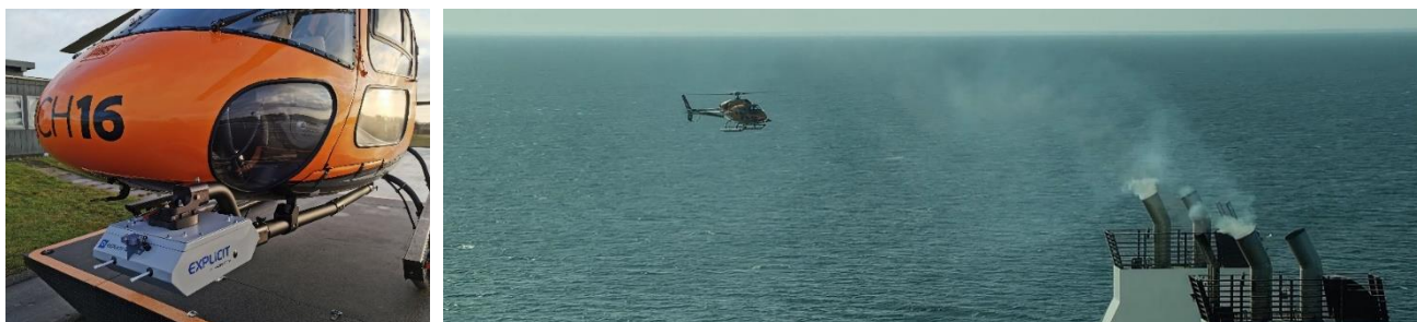
The Explicit Mini Sniffer System mounted on an AS355 helicopter, and a scrubber vessel being sampled in Danish waters. Photos: Explicit ApS / Charlie 9 Helicopters ApS.
