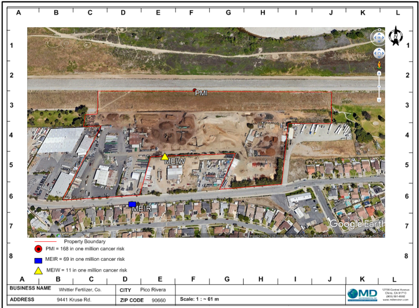
Figure 2. Location of the PMI, MEIW, and MEIR calculated based on the health risk assessment.
