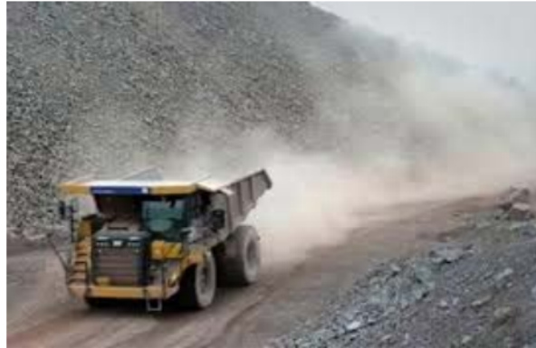
Figure 1-6 Fugitive Dust from Off-Road Hauler
