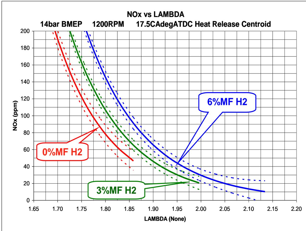
Lambda at the limit of combustion stability was observed to be as follows:
