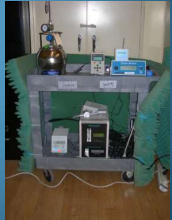
Mobile station monitoring indoor/outdoor concentrations of PM
